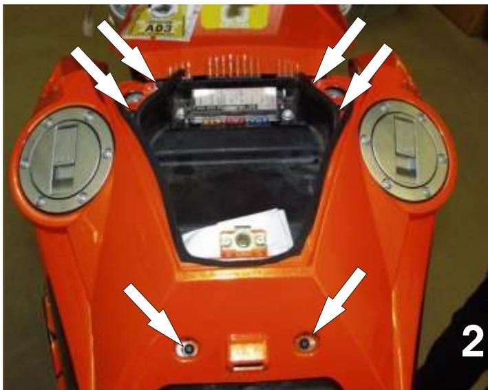
Turn off both gas lines. Loosen the screws holding the right tank, remove it and disconnect the hoses.
